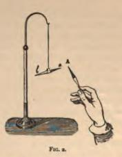
Magnetism of Broken Magnets.—If a bar that has been magnetized be broken in the middle, each half will have two poles and a neutral point in the centre. If one of these halves is broken in the middle, each half will be found to have two poles and a neutral line. If one of these parts in turn be broken, each half will again be found to be a complete magnet, with two poles and a neutral line, and so on as long as we can carry the division.
